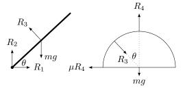
Taking moments around the hinge,  $R_3 = mg \cos \theta$ . Resolving vertically for the block,
